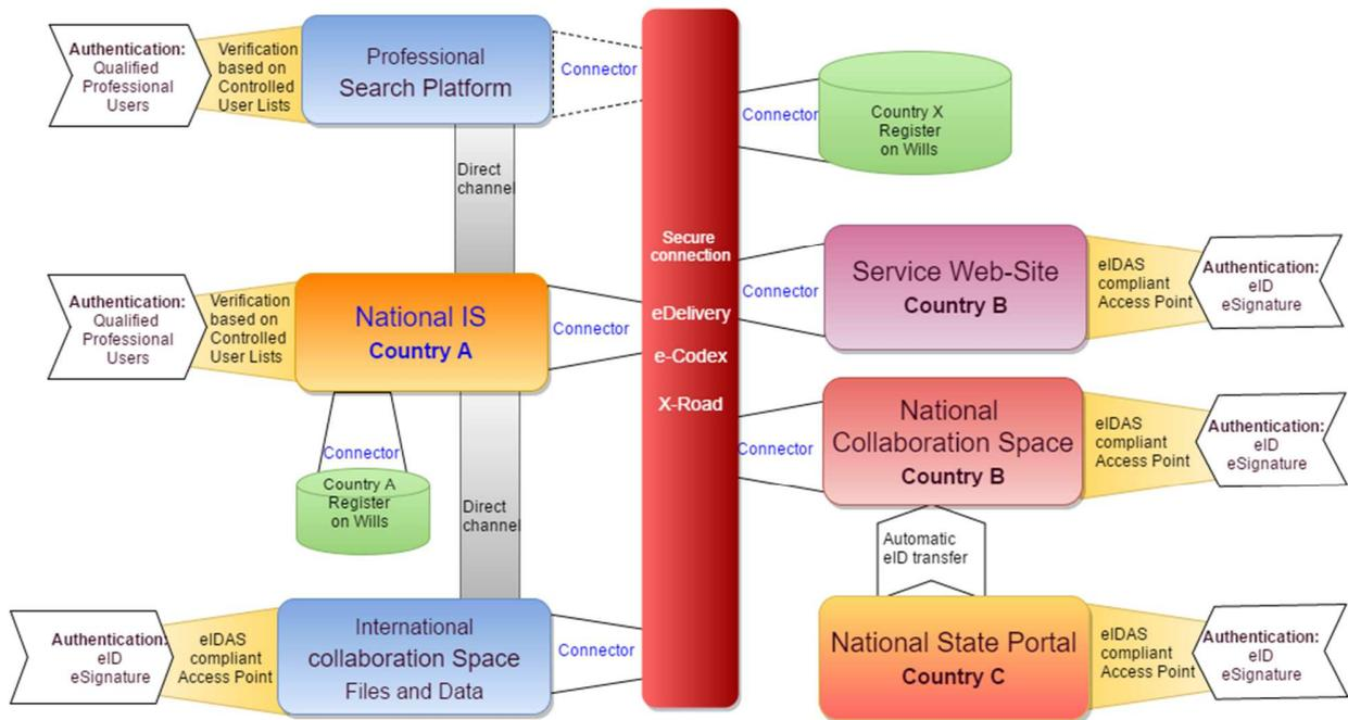
Figure 2. Overview of possibilities for connecting information systems over secure network connections, and for authenticating users of the network of interconnected systems.
